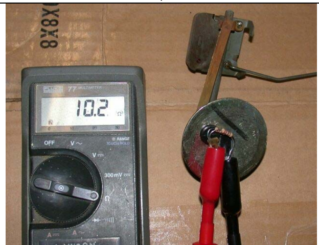
Sending unit “Full” with 135 Ohm parallel resistor
