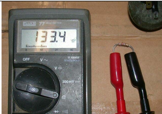
Two (2) 270 Ohm resistors in parallel = 135 Ohms
