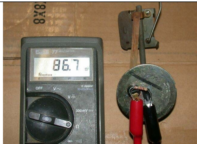
Sending unit “Empty” with 135 Ohm parallel resistor.
